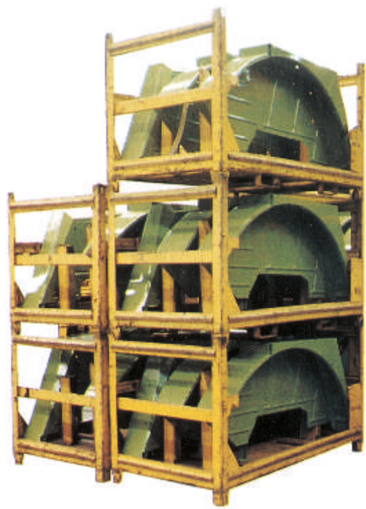
Transport and storage frame for prefabricated parts as intermediate storage
